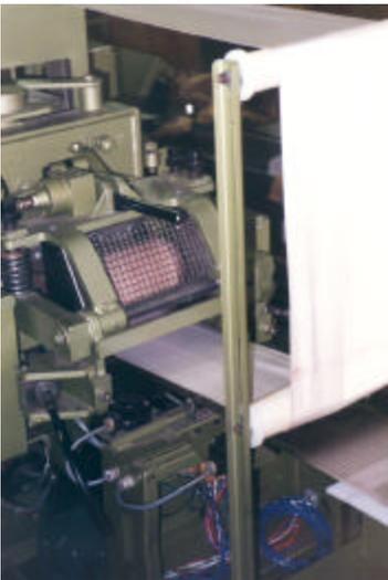
leakage, the head was under a tremendous amount of pressure. On each pass of the counterband splice through the pressure rolls, the additional thickness of the counterband splice combined with the excessive head pressure, was actually making the small indentions into the stainless steel. The stainless steel belt failed prematurely due to crack propagation down the line of indentions created by the splice in the counterband.
